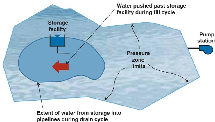
replacing the standpipe with an elevated tank reduced water age by almost 40%, from approximately 415 hours (17 days) to approximately 260 hours (11 days).
