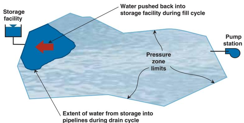
**FIGURE 4** Movement of water in system for a storage facility within the demand area
