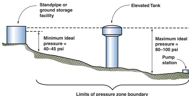
standpipe or ground storage reservoir generally can be constructed more economically, which is one reason that standpipes and ground storage reservoirs are often selected in lieu of elevated tanks. However, standpipes and ground storage reservoirs may be susceptible to high
