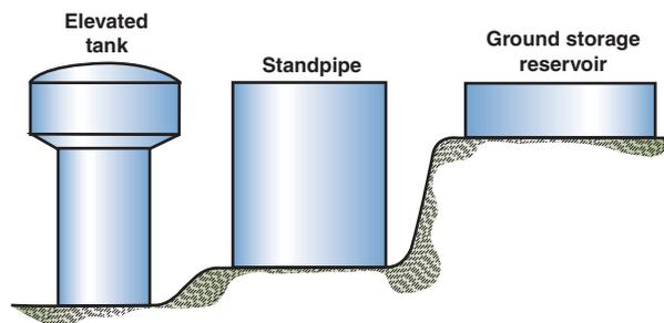
tems can be sited at higher elevations, allowing for gravity service to all or portions of a service area or pressure zone” (SEWRPC, 2006). A technical brief on storage facilities issued by the National Drinking Water Clearinghouse included this note: “In hilly areas, however, it may be more advantageous to select the highest point for construction of an elevated tank which may lie at one end of the area instead of the center” (Bhardwaj, 2001).
