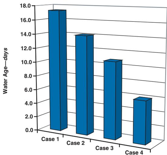
*Case 1 = standpipe outside demand area, 15-ft fluctuation; case 2 = standpipe outside demand area, 20-ft fluctuation; case 3 = elevated tank outside demand area, 15-ft fluctuation; case 4 = elevated tank within demand area, 15-ft fluctuation*
