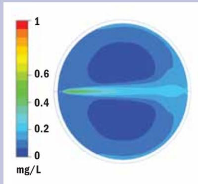
in temperature and water age with each fill-and-draw cycle. Deep cycling this tank 50 percent won't correct the problem. The tank will short-circuit because freshwater is pulled from the bottom of the tank, leaving poor-quality water in the top of the tank. This problem can occur in all styles of storage tanks, but particularly in standpipes, because of their depth.
