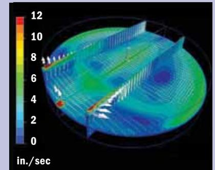
last. To prevent short-circuiting, this tank needs two outlet pipes—one in each semicircular low-velocity area. With a properly designed passive mixing system, however, the location of the outlet pipe isn't critical because the entire water volume will be mixed and homogenous.
